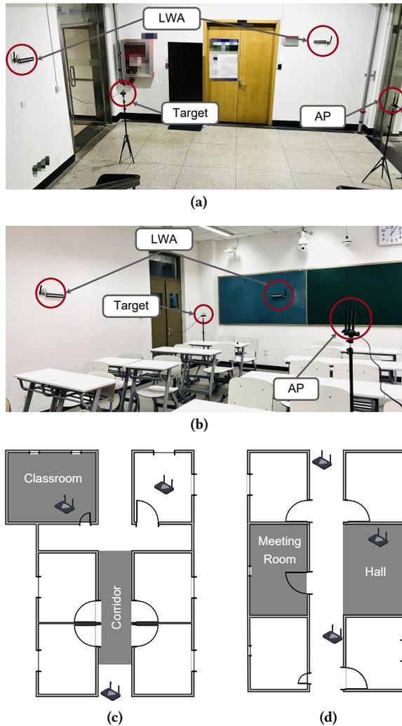
**Figure 12: Experimental scenarios and deployment:** (a) The hall scenario; (b) The classroom scenario; (c) The APs' deployment in the corridor and the classroom; (d) The APs' deployment in the hall and the meeting room.
