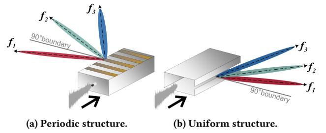
Figure 6: Typical structures of leaky wave antenna<sup>3</sup>.
